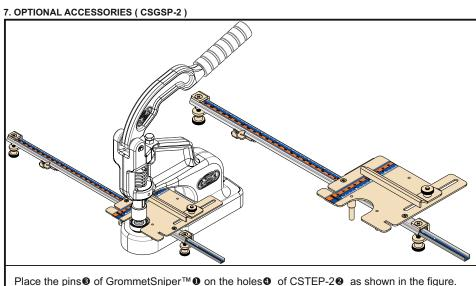
Place the pins● of GrommetSniper™● on the holes● of CSTEP-2● as shown in the figure. Gently tighten it manually. After making sure that there is no tightness or irregular connection, tighten the fixing screw● with a Philips head screwdriver.
